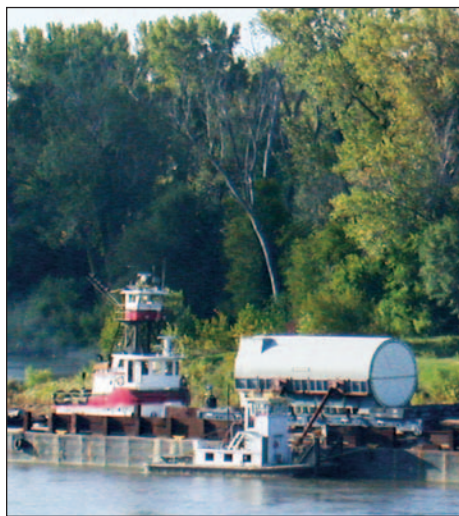
A barge carrying Cooper Station’s generator stator docks next to a boat ramp on its way to the plant.
