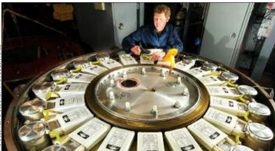
Sandia researcher Bill Fowler tests circuits on a device able to produce large electrical impulses for the Z.
