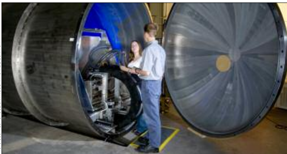
Daniel Maierhafer and Katherine Atchley, research associates in the Neutron Scattering Sciences Division at Oak Ridge, examine a neutron scattering tank installed at the High Flux Isotope Reactor.
